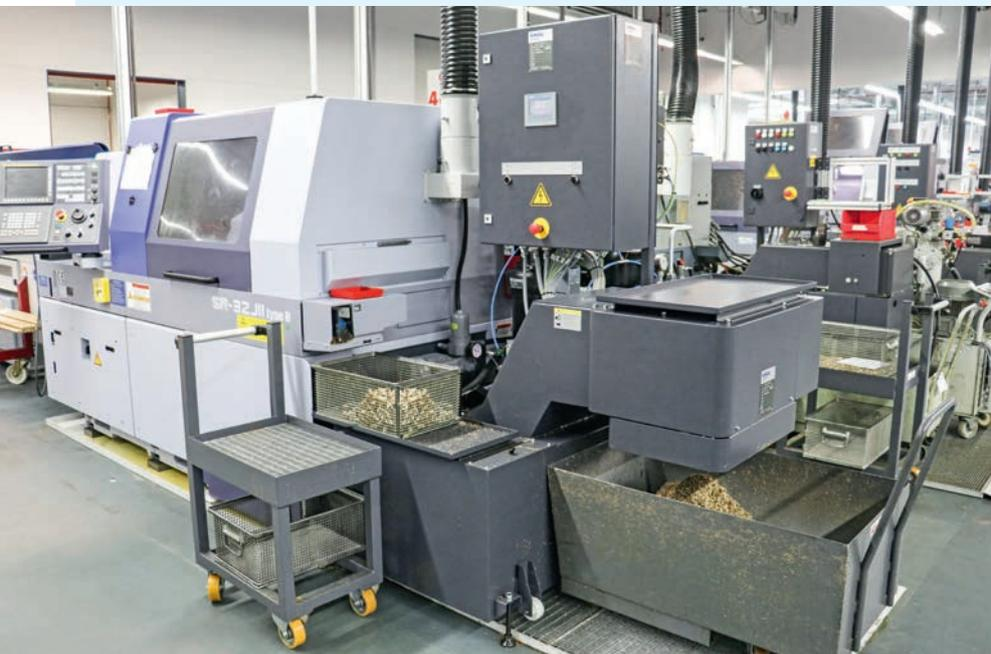
For years, Gerland has had KNOLL equip automatic lathes with a permanently installed combination of chip conveyors, filtration systems and high-pressure pumps.
