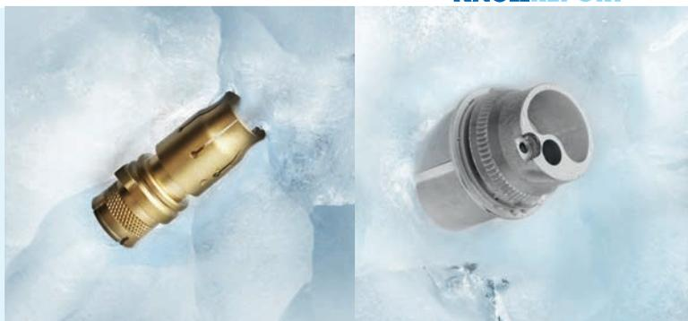
A typical Gerland component for automation technology made of brass (left) and a special aluminium alloy (right). Machining requires a stable machine design. A cooling lubricant supply of more than 80 bar increases the surface quality and service life considerably.
